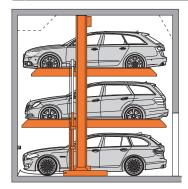
Before lowering the platforms, the vehicle parked in the lower parking space must be driven off!
